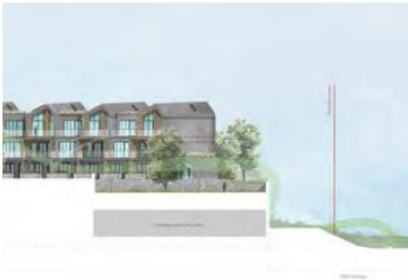
Figure 7.7: Extended cross section AA (CD2.005) through northern site boundary – illustrating 6m high retaining wall containing northern edge of hotel service area (equivalent height of two storeys)
