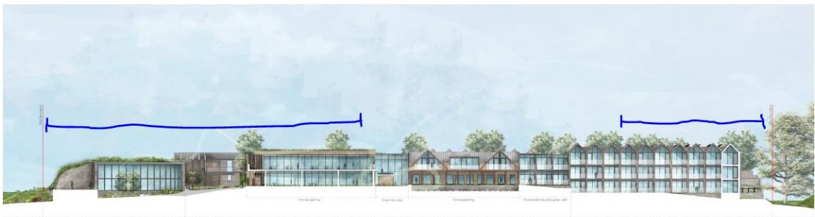
Figure 7.4: Section AA from DAS Addendum (CD 2.014) – blue lines indicate length of existing frontage which is currently single storey or undeveloped (see photos above). This illustrates the increased prominence that built form will have along Ferry Road. Section also illustrates that the spa buildings is the same height as the two storey hotel building – ie it is not single storey building (as stated in the DAS)
