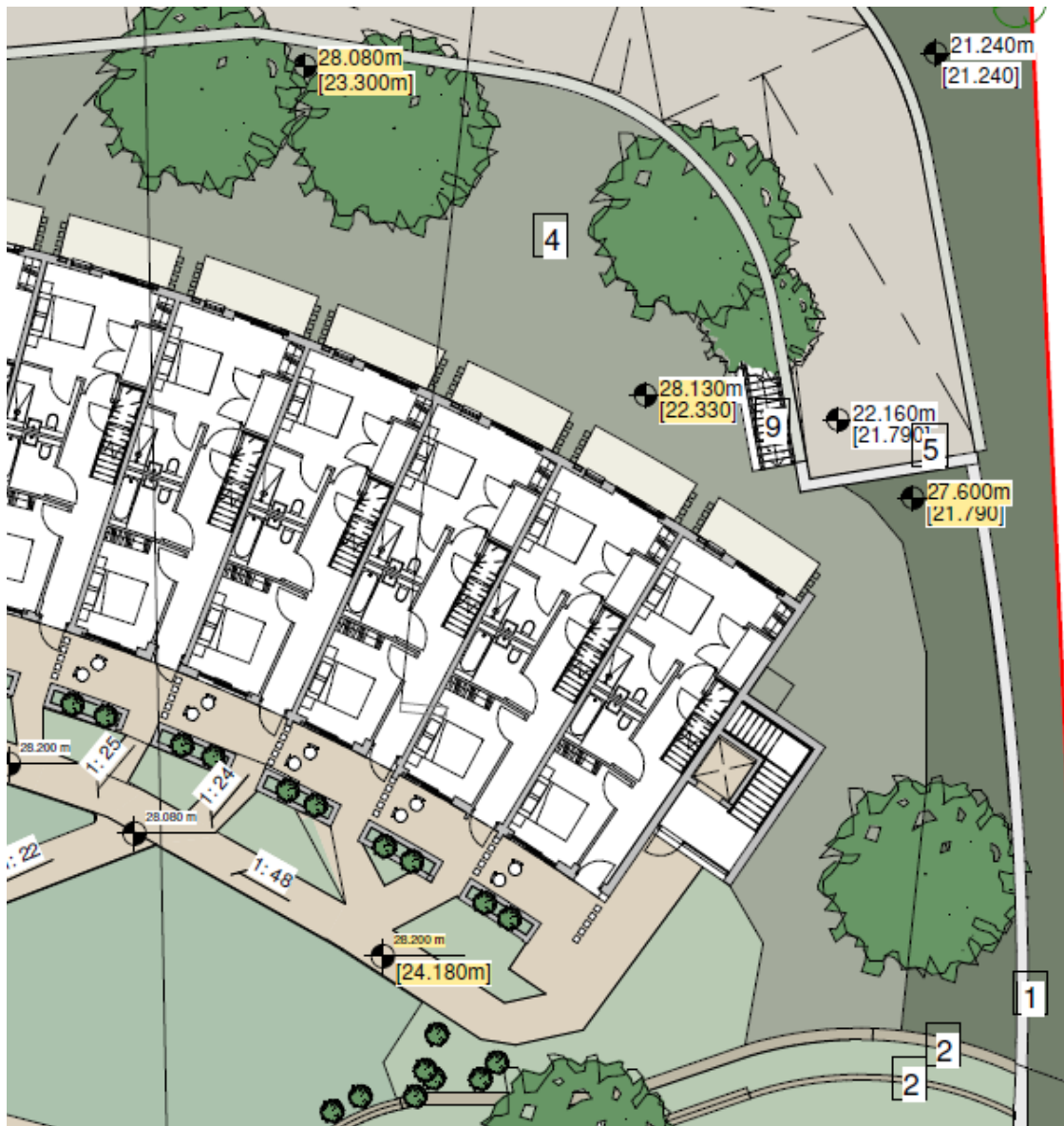
Figure 6.1: Extract of Dwg 20002 P011 (CD2.003) – illustrating existing (in square brackets) and proposed levels (without brackets) and showing proposal to raise levels by 4 – 6m in north-west part of the Site
